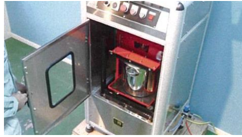
2. Cover a container with a lid and set the container to VP series mixer
